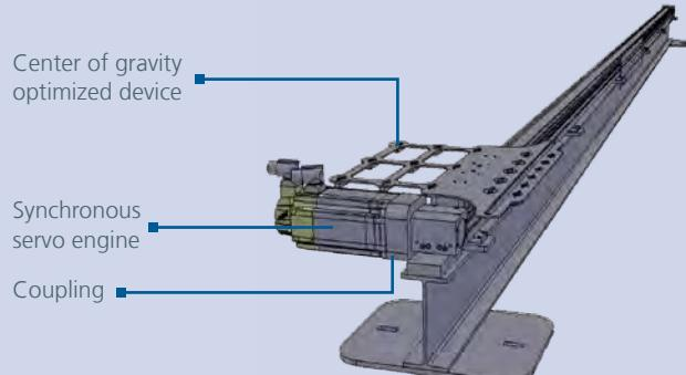
The system design is modular and achieves feed rates of up to 600 m/min according to the "moving workpiece" concept.
