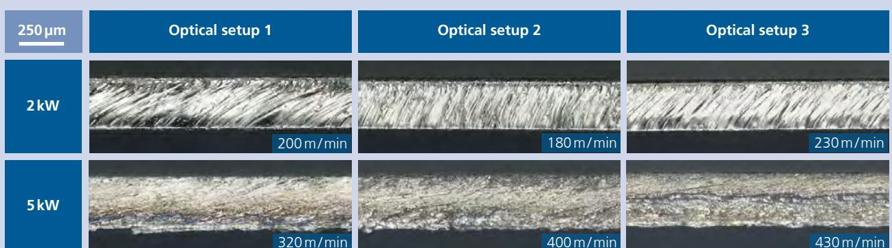
Depending on the selected optical setup and laser power, different cutting speeds and cut qualities can be achieved.
