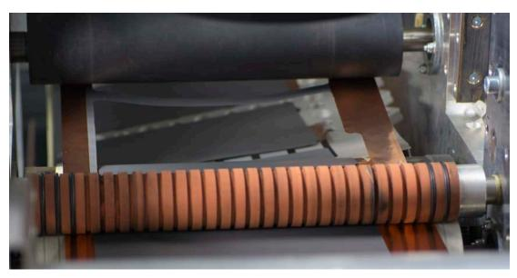
Electrode packaging with laser "on the fly" © Fraunhofer IWS Dresden
