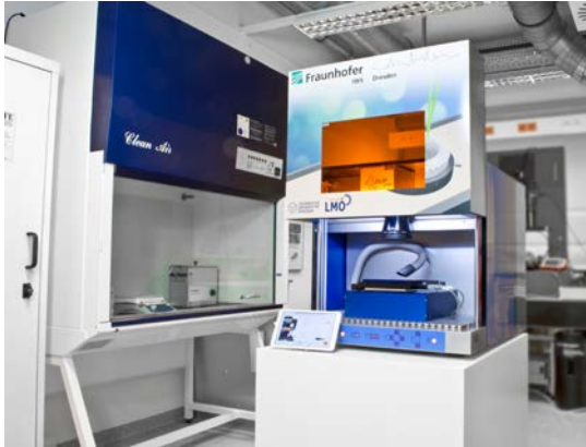
Compact system for surface structuring by means of scanner-based direct laser interference patterning © Fraunhofer IWS Dresden
