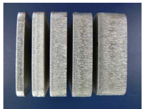
Fig. 3: Cutting edge quality of aluminum, (left: material thickness 4 - 12 mm) and stainless steel samples (right: material thickness 4 - 15 mm)
