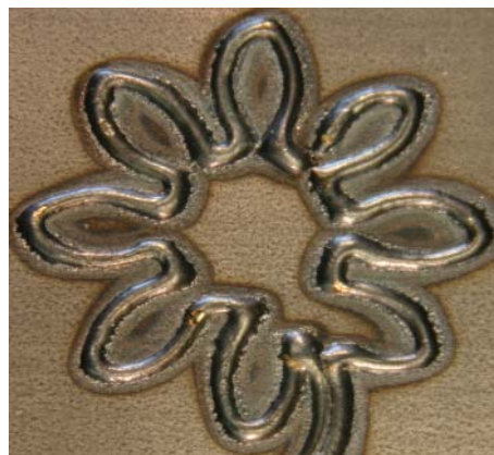
Fig. 2: Laser contour buildup weld with central wire feed (1.3 mm track width)
