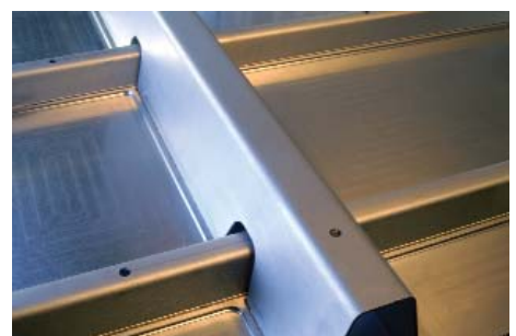
Completely laser welded integral structure for aircraft fuselages in closed profile design (demonstrator)
