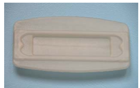
Fig. 4: Injection molded part, manufactured with the tool insert as shown in Fig. 3
