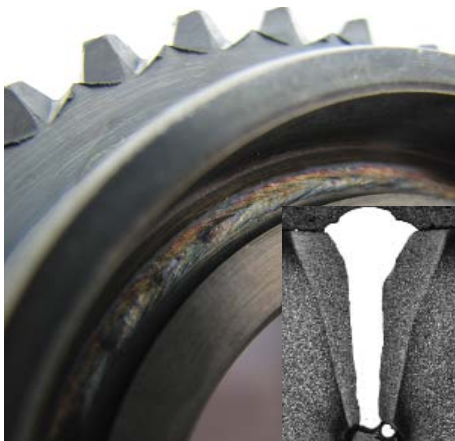
Fig. 2: Carbo-nitrided part after combined removal and welding process
