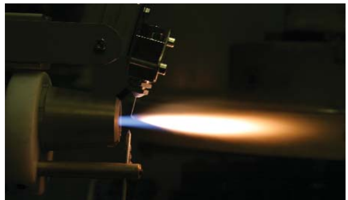
Fig. 2: HVOF flame jet with external injection of an alcoholic suspension
