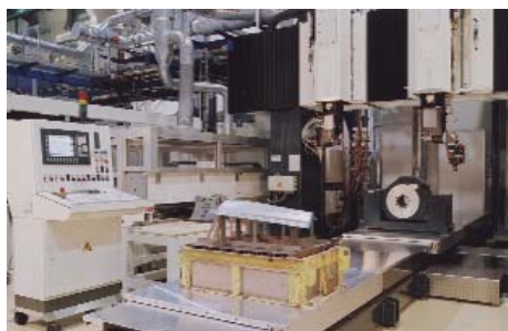
High-speed 3D laser cutting system with linear drives
