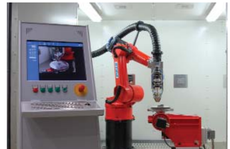
Robot system with 6 kW laser for laser buildup welding
