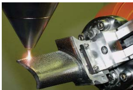
Repair of gas turbine blades through buildup welding with high power diode lasers
