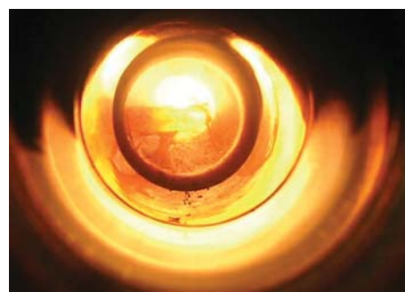
Arc synthesis of filaments made of carbon nanotubes
