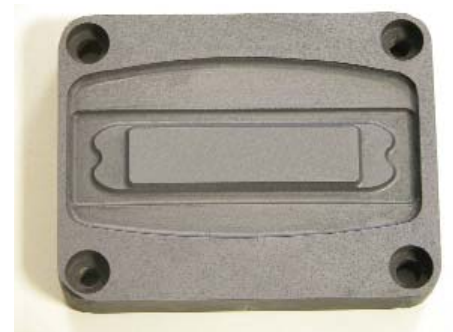
Fig. 3: Completed tool insert after removal of the positive model and finishing
