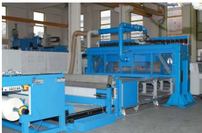
Laser system "Contilas 2500" for airbag fabrication
