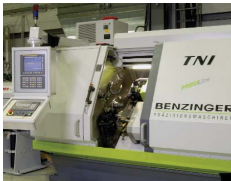
Integration of the laser beam hardening process in a lathe, example: hydraulic components for Bosch-Rexroth
