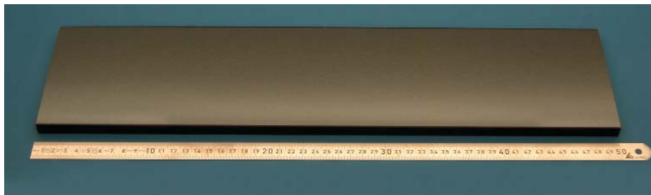
Fig. 2: DLC coated glass plate with dimensions of 500 x 100 mm 2
