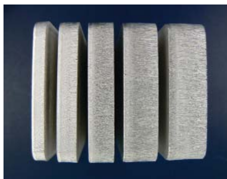
Fig. 3: Cutting edge quality of aluminum, (left: material thickness 4 - 12 mm) and stainless steel samples (right: material thickness 4 - 15 mm)
