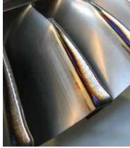
Left: Induction-assisted additive manufacturing of a component. Right: Laser cladding is a well established technology for the repair of turbine blades.
