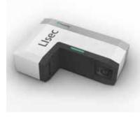
The Lisec (derived from "Light Section") powder nozzle measuring system automatically measures the geometry of the powder stream cone prior to the process. For this purpose, a measurement laser illuminates the powder stream as it leaves the nozzle. The number of measurement levels is freely definable. A camera is mounted at right angles to it. This records light sections through the
