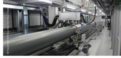
This customized facility has been coating off-shore hydraulic cylinders around the clock since 2016 using 20kW of laser power and induction.
