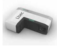
The Lisec (derived from "Light Section") powder nozzle measuring system automatically measures the geometry of the powder stream cone prior to the process. For this purpose, a measurement laser illuminates the powder stream as it leaves the nozzle. The number of measurement levels is freely definable. A camera is mounted at right angles to it. This records light sections through the
