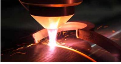
Combining laser cladding and induction not only enables cracksensitive base materials to be coated smoothly, but also significantly increases the application rate.
