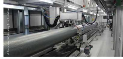
This customized facility has been coating off-shore hydraulic cylinders around the clock since 2016 using 20kW of laser power and induction.
