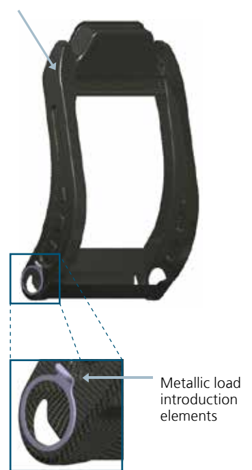
HPCi®-joined seat frame hybrid composite structure.
