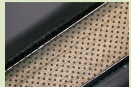
Tribologically efficient laser micro structures on a motor component
